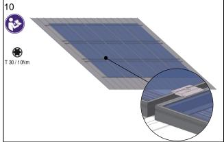
18.1 Appendix 5 Installation of sheet metal seam clamp MSP-PR-SC 70 on a copper roof with a stainless steel saddle MSP-PR-SCC 40
